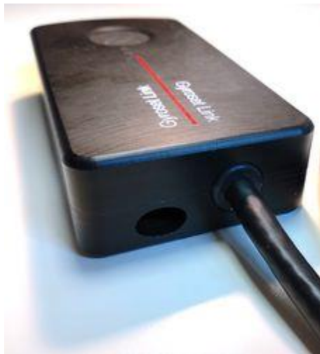
The two interfaces of the Link (on the left the oval shaped data connector)
