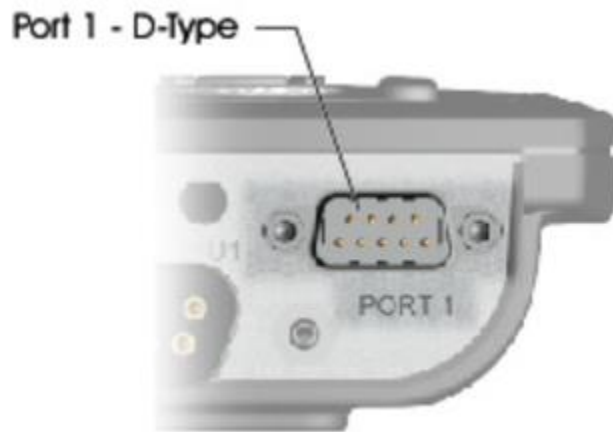
Omni Port-1 D-type connector
