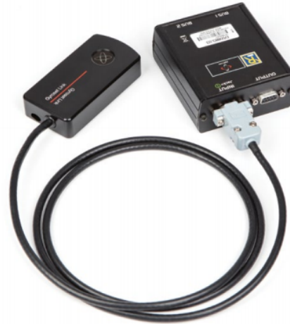
Connecting the GyroSet™ Link to IOM
